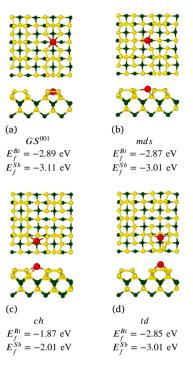
Fig. 9. Stable adsorption sites on the GaAs (001) surface. Yellow, green and red spheres represent As, Ga and Bi/Sb atoms, respectively.
