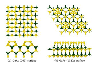
**Fig. 1.** Top and side views of the supercells used for the modeling of (a) the GaAs (001) surface and (b) the GaAs (111)A surface. For clarity, only the topmost layers are represented. Yellow and green spheres represent As and Ga atoms, respectively.
