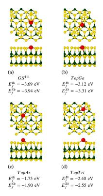
Fig. 10. Stable adsorption sites on the GaAs (111)A surface. Yellow, green and red spheres represent As, Ga and Bi/Sb atoms, respectively.
