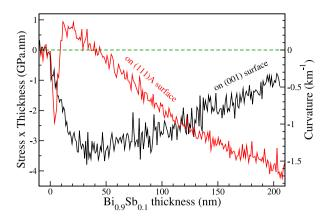
**Fig. 11.** Stress×thickness product (left axis), or wafer curvature (right axis), as a function of the deposited  $Bi_{0.9}Sb_{0.1}$  thickness on GaAs (001) (black line) or on GaAs (111)A (red line), at 215 °C (Bi flux of  $4 \times 10^{-7}$  Torr and Sb flux of  $5 \times 10^{-8}$  Torr for both growths).
