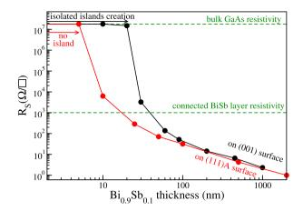
Fig. 3. Variation of the sample resistivity for different  ${\rm Bi}_{0.9}{\rm Sb}_{0.1}$  thicknesses on the GaAs (001) (black) and GaAs (111)A (red) surfaces.
