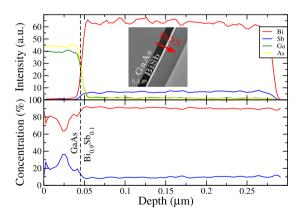
**Fig. 8.** Variation of the energy dispersion spectroscopy (EDS) intensities for each atom type (top panel) while crossing the BiSb grain. The beam path is represented by the red arrow on the insert transmission electron microscopy (TEM) panel. The calculated Bi and Sb concentrations (bottom panel) are calculated from there respective intensities.
