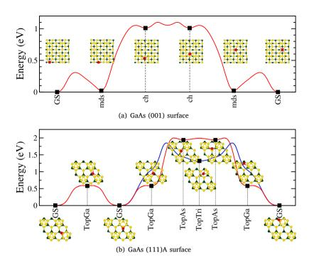
Fig. 4. Minimum energy pathways of the Bi atom between the ground state positions above the (a) GaAs (001) and (b) GaAs (111)A surfaces. Red ball represent the adsorbed Bi atom.
