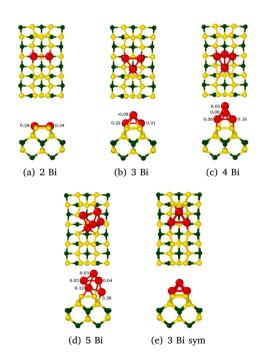
**Fig. 6.** Most stable atomic configurations of the agglomeration of two to five Bi atoms on the GaAs (001). Structures 3 and 5 can exist symmetrically, and an example is given for structure 3 panel 6(e). Variation of Bader charge is given on each adsorbed Bi atom in reference to the value of Bi in its pseudopotential.
